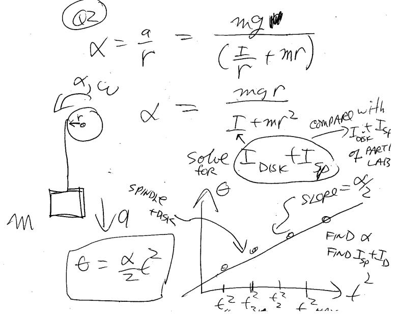
GRAPH THE LINE AND FIND THE SLOPE OF  $\theta$  vs.  $t^2$ .
